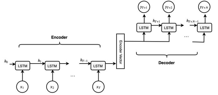
Fig. 5. LSTM Encoder-Decoder.
