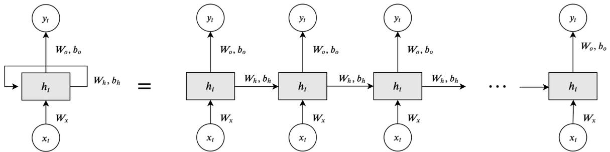
Figure 4.6: Recurrent Neural Network structure.
