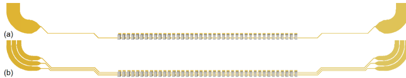
Figure 5.1.1: Stimulation and Sensing design; (a) 1 turn, (b) 3 turns.
