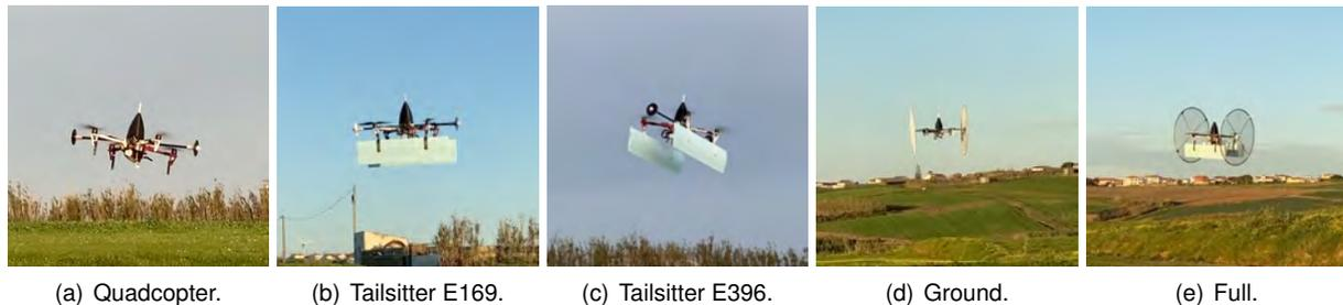
Figure 5.9: Different flight configurations in hove flight.
